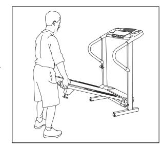
Move your right hand to the position shown and hold the treadmill firmly. Using your left hand, pull the latch knob to the left and hold it. Raise the treadmill until the frame passes the latch pin. Slowly release the latch knob. Make sure that the frame is securely held by the latch pin.
